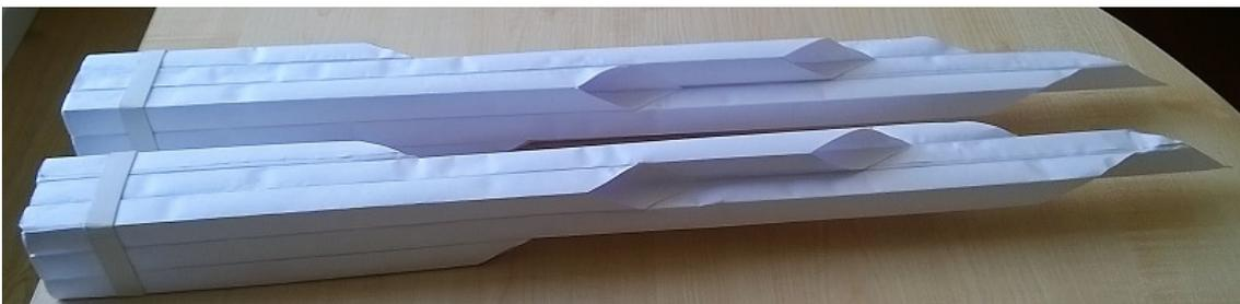
Section 3 and 4. The paper waveguides are nine for geometric reasons. Each paper wave guide is square and has a 20x20mm section, the lengths are between 100 and 700 mm. The nine waveguides form a 3 x 3 square matrix.
